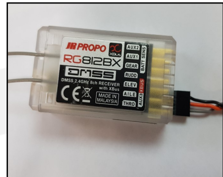
Please note cable polarity on a RG812BX
