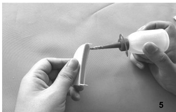
Fig. 5 - Glue the servo fairing.
