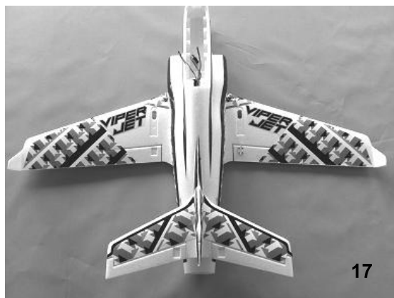
Fig. 17 - The photo shows the finished view after gluing the vertical stabilizers in place.
