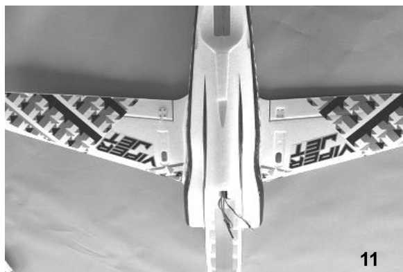
Fig.11 - The photo shows the finished view after gluing the wings in place.
